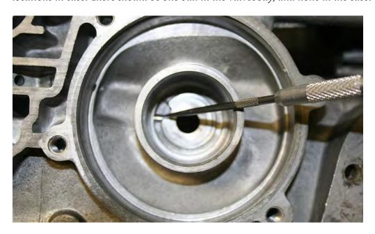
11. Flat file or wet stone entire channel passage area of case - absolutely no high spots or burrs allowed especially at area shown below.
