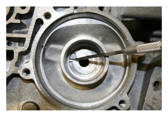
15. Flat file or wet stone entire channel passage area of case - absolutely no high spots or burrs allowed especially at area shown below.
