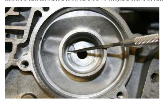
10. Flat file or wet stone entire channel passage area of case - absolutely no high spots or burrs allowed especially at center support case area shown below.
