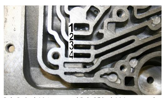
Brake On: Lands 3 & 4 are connected. Brake Off: Lands 2 & 3 are connected. Ensure solenoid plunger completely bottoms on solenoid back when stroked. Shims on bracket bolt may be needed when there is a shim on the solenoid.
