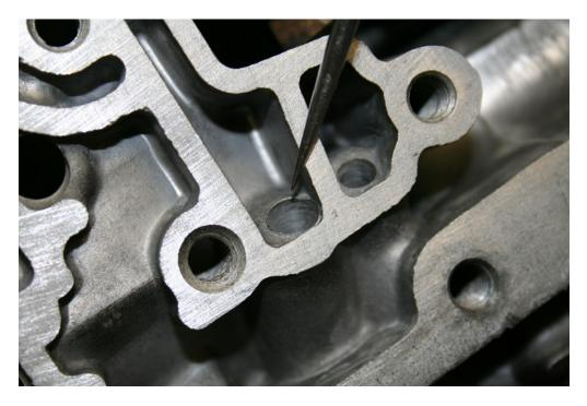
5. Install band servo plug (steel) as shown below.
