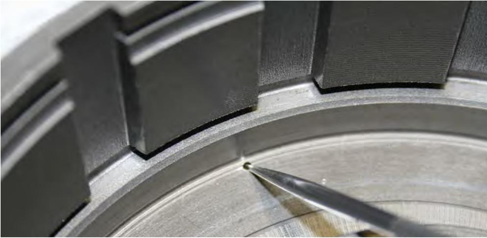
3. Replace piston lip seals and discard center seal in drum. Be sure to install both seals on the piston, and none in the drum.
