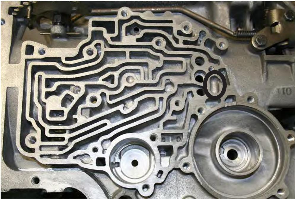
11. DO NOT install any gaskets on the case or valvebody! Install valvebody. Start all valvebody bolts before tightening! Torque to 15 ft-lbs (5/16" bolts) and 10 ft-lbs (1/4" bolts).
