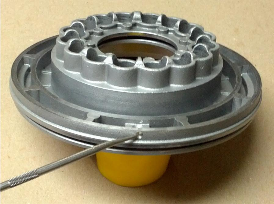
8. Install piston in drum and replace every other return spring with the 8 new included return springs, and install new clutches.
