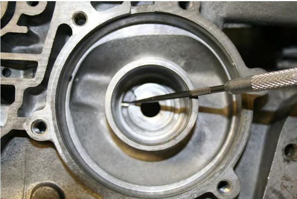
15. Flat file or wet stone entire channel passage area of case - absolutely no high spots or burrs allowed especially at area shown below.
