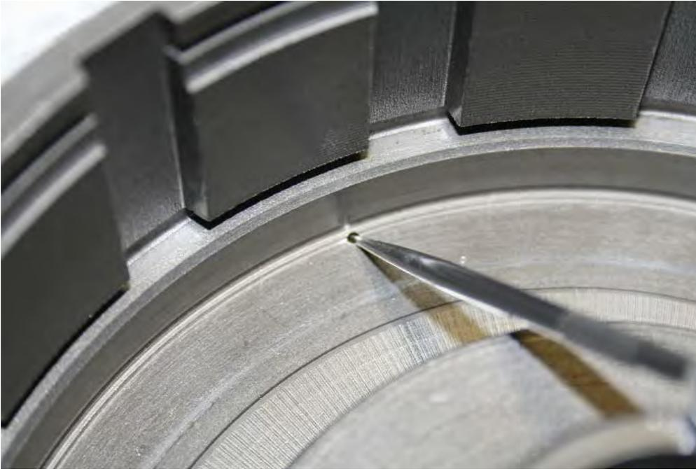
3. Replace piston lip seals and discard center seal in drum. Be sure to install both seals on the piston, and none in the drum.
