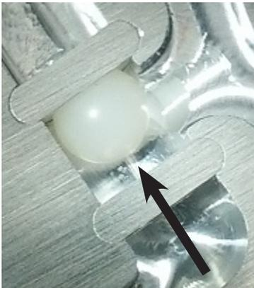
21. DO NOT install any gaskets on the case or valvebody! Install transbrake valve body. Start all valve body bolts before tightening!
