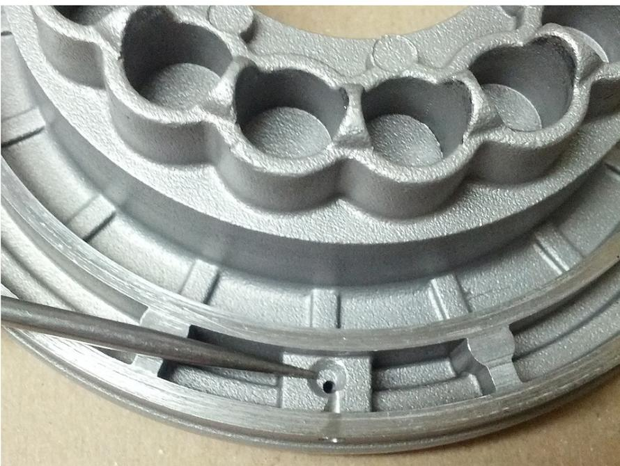
7. Drill 1/8" hole in forward drum piston at outer edge and inline with .040" hole, as shown below.
