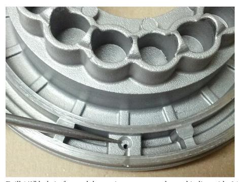
7. Drill 1/8" hole in forward drum piston at outer edge and in line with .040" hole, as shown below.
