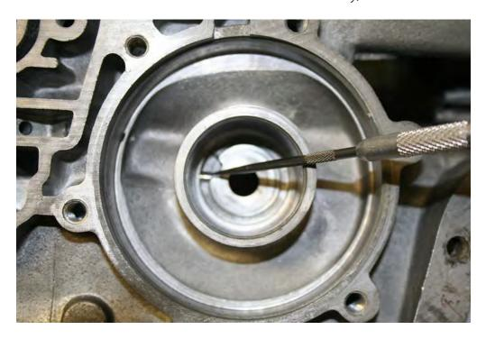
14. Flat file or wet stone entire channel passage area of case - absolutely no high spots or burrs allowed especially at area shown below.
