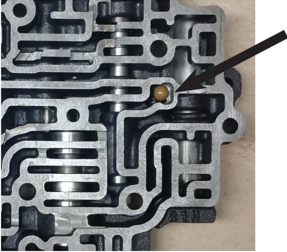
17. Install transbrake valve body with included separator plate.
