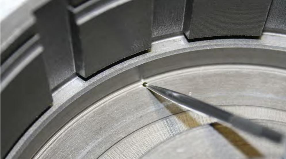
3. Replace direct clutch apply piston lip seals and discard the center seal in the drum.
