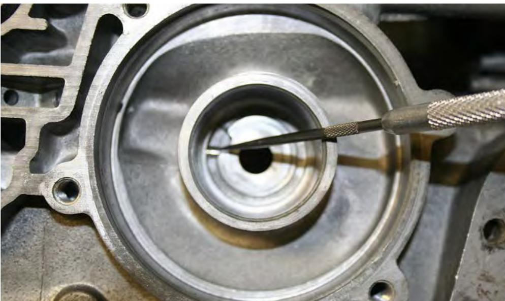
10. Flat file or wet stone entire channel passage area of case - absolutely no high spots or burrs allowed especially at center support case area shown below.
