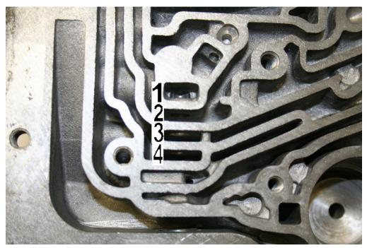
Brake On: Lands 3 & 4 are connected. Brake Off: Lands 2 & 3 are connected. Ensure solenoid plunger completely bottoms on solenoid back when stroked. Shims on bracket bolt may be needed when there is a shim on the solenoid.
