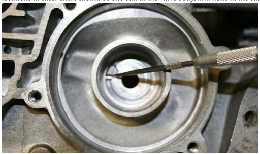
11. Flat file or wet stone entire channel passage area of case - absolutely no high spots or burrs allowed especially at center support area shown below.
