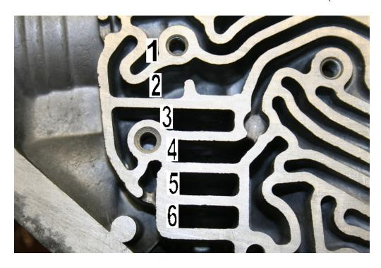
Brake ON: Lands 3 & 4 are connected. Brake OFF: Lands 4 & 5 are connected.
